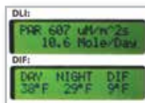
Displays Daily Light Integral (DLI) and Day/Night Temperature Difference on the LCD
