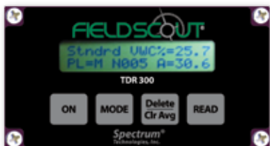
LCD display shows current measurement, rod length, number of readings, and running average
