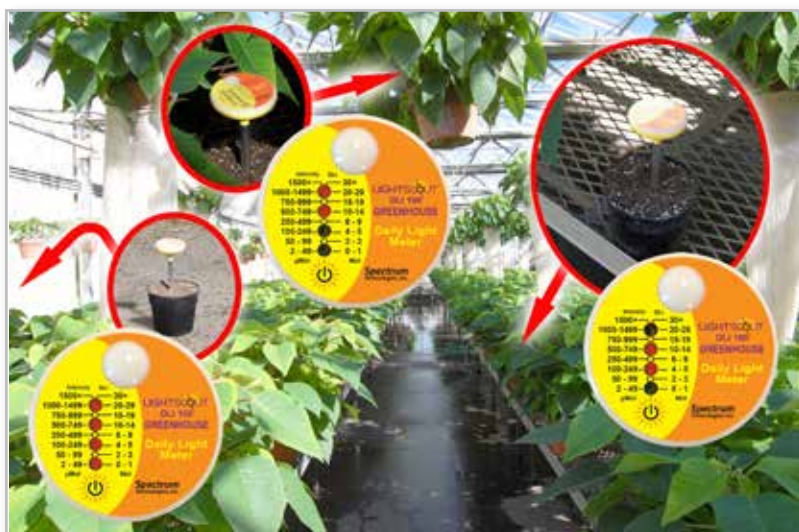
Greenhouse growers can position the meters throughout the greenhouse, as well as outside, to compare differences in light levels and the effect on plant growth and quality.
