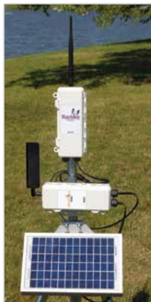
DataScout Model 110 Modem mounted with a WatchDog Retriever
